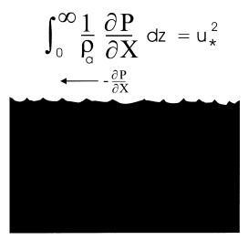
FIG. 1. Idealized experimental setup. A uniform, infinitesimal, horizontal pressure gradient is applied throughout a semi-infinite gas with no buoyancy stratification. This integrated momentum source is balanced by a momentum flux into the water. A slight slope of the water surface provides the net momentum sink needed to balance the atmospheric source.
