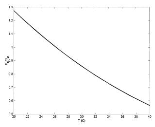
FIG. 3. The ratio of the enthalpy exchange coefficient to the drag coefficient, each based on the gradient wind, according to (27). The ratio is plotted as a function of the undisturbed air temperature.
