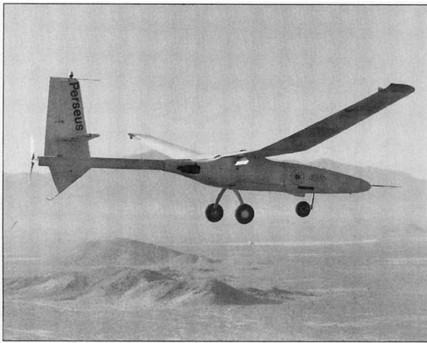
FIG. 1. The Perseus Proof of Concept aircraft. The structural and electronics development testbed for the Perseus family, this aircraft completed its initial flight testing in November 1991. The plane has an 18-m wingspan and a gross weight of 430 kg.
