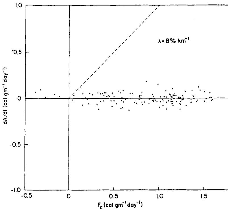
Figure 3. Observed rate of change of cloud work function  $A$  (ordinate) plotted against rate of change of  $A$  due to large-scale processes only, for a particular value of the entrainment rate. (From Arakawa and Schubert (1974).)
