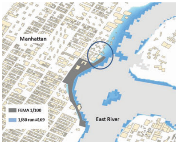
Fig. 12. The current FEMA 1/100 flood zone for a part of Manhattan and, shown in blue, the extent of simulation run #169 with a probability of 1/80.
