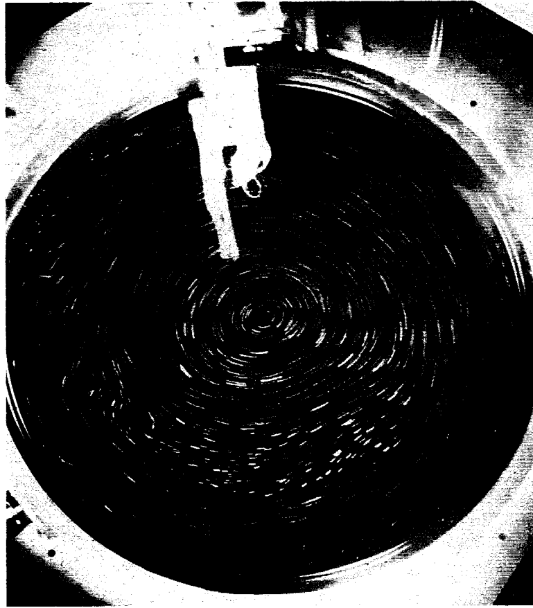
FIG. 6. Motion at free surface of water in differentially heated dishpan rotating at 1.9 rpm, after statistically steady state has been attained. Radius 19.5 cm, depth of water 4.2 cm. Photo through courtesy of D. Fultz.
