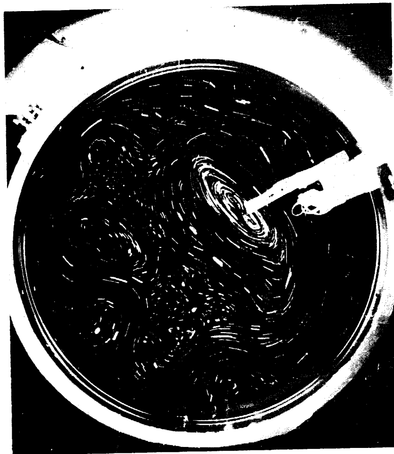
FIG. 7. Motion at free surface of water in dishpan heated as in Figure 6, rotating at 3.8 rpm, after statistically steady state has been attained. Photo through courtesy of D. Fultz.
