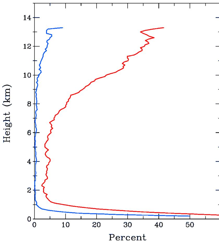
Figure 1. Frequency of  $R_B < 0.25$  (cyan) and  $R_B < 1$  (red) for all G-IV dropsondes within 1500 km of the storm center.
