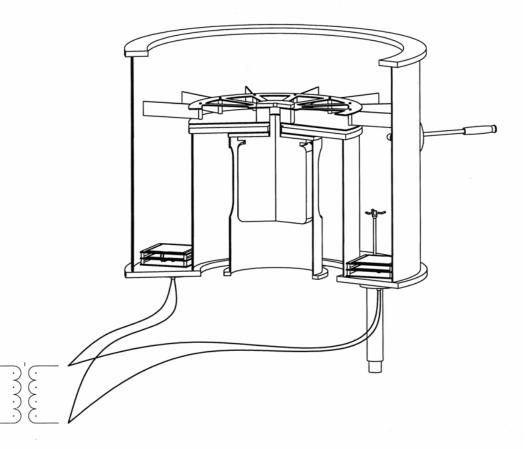
Figure 1.4: Multiple heating elements inside the wind wave tank. A transformer provides power at 24 Volts.
