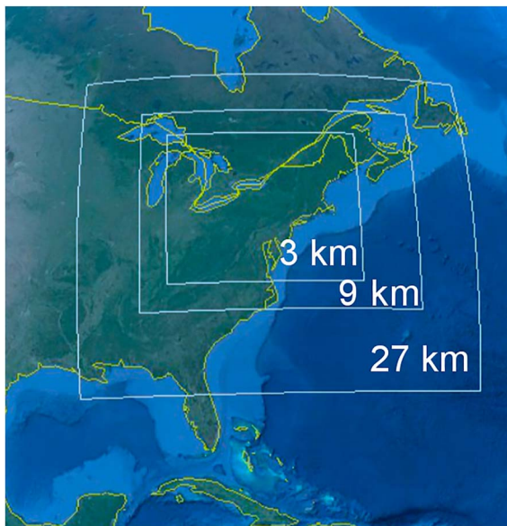
Figure 1. WRF simulation domain, three nested grids of 27-, 9-, and 3-km horizontal resolution, used in this study.
