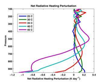
Figure 6. Perturbation net radiative heating rates in response to an instantaneous reduction of specific humidity of 20% from the RCE states for SSTs ranging from 25 to 45°C.
