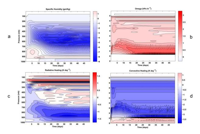
Figure 3. Time-height sections of perturbations from the RCE state of (a) specific humidity, (b) omega, (c) radiative heating, and (d) convective heating. Time is in days after reinitialization from the RCE state under WTG. The surface temperature in this case is 40°C.
