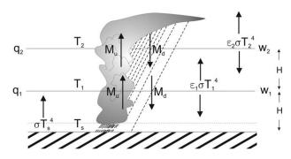
Figure 1. The two-layer model. Surface temperature and the temperatures of each layer are specified and constant. The emissivities,  $\varepsilon$ , updraft and downdraft mass fluxes,  $M_u$  and  $M_d$ , large-scale vertical velocities, w, and specific humidities, q, are variable. The vertical arrows depict the convective and radi-
