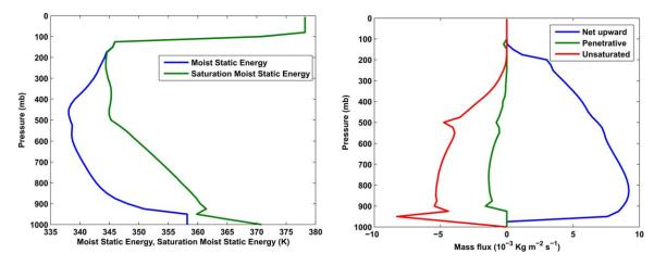
Figure 2. Vertical profiles of (left) moist static energy and (right) convective mass fluxes at equilibrium in the control simulation, for which the SST = 30°C. Moist static energy is shown in blue, and saturation moist static energy is shown in green. The convective mass fluxes are composed of buoyant updrafts (blue), penetrative downdrafts (green), and a precipitationdriven unsaturated downdraft (red).
