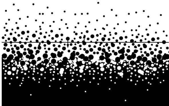
FIG. 2. Momentum and enthalpy transfer through an emulsion. Spray droplets are ejected upward and accelerate toward the free stream velocity, absorbing momentum from the atmosphere.
