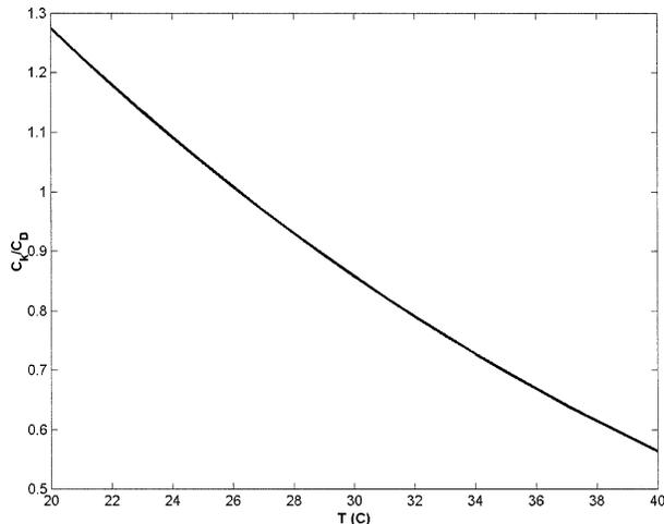
FIG. 3. The ratio of the enthalpy exchange coefficient to the drag coefficient, each based on the gradient wind, according to (27). The ratio is plotted as a function of the undisturbed air temperature.
