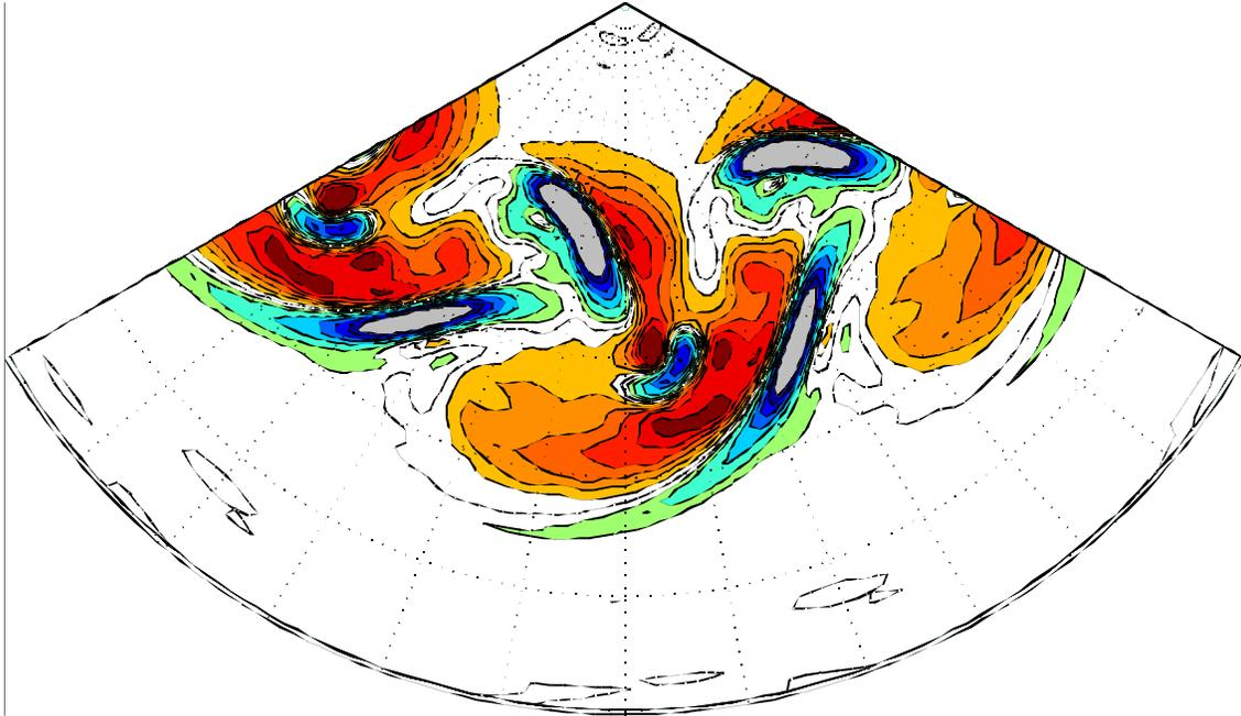
**Figure 2: Distribution of vertical velocity over a third of the Northern Hemisphere in a primitive equation model simulation, in which condensation is represented by applying a reduced static stability to upward moving air. Cool colors represent upward motion; warm colors represent downward motion. (Model designed by and figure courtesy of Tieh Yong Koh.)**
