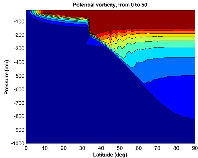
**Figure 1: Potential vorticity in a radiative-slantwise convective equilibrium state, with an assumed isothermal stratosphere. The troposphere is assumed to be neutral to slantwise moist convection and to have vanishing zonal wind at the surface; the wind distribution above the surface is determined from the thermal wind equation.**
