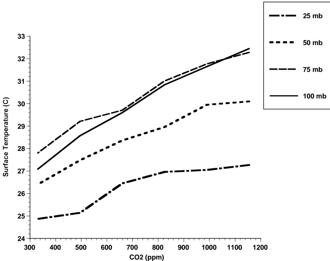
Figure 6: Dependence of surface temperature in radiative-convective equilibrium on atmospheric CO2 content, for four different vertical resolutions, using the convection scheme described by Emanuel and Zivkovic-Rothman (1999) and the radiation scheme of Chou et al. (1991).
