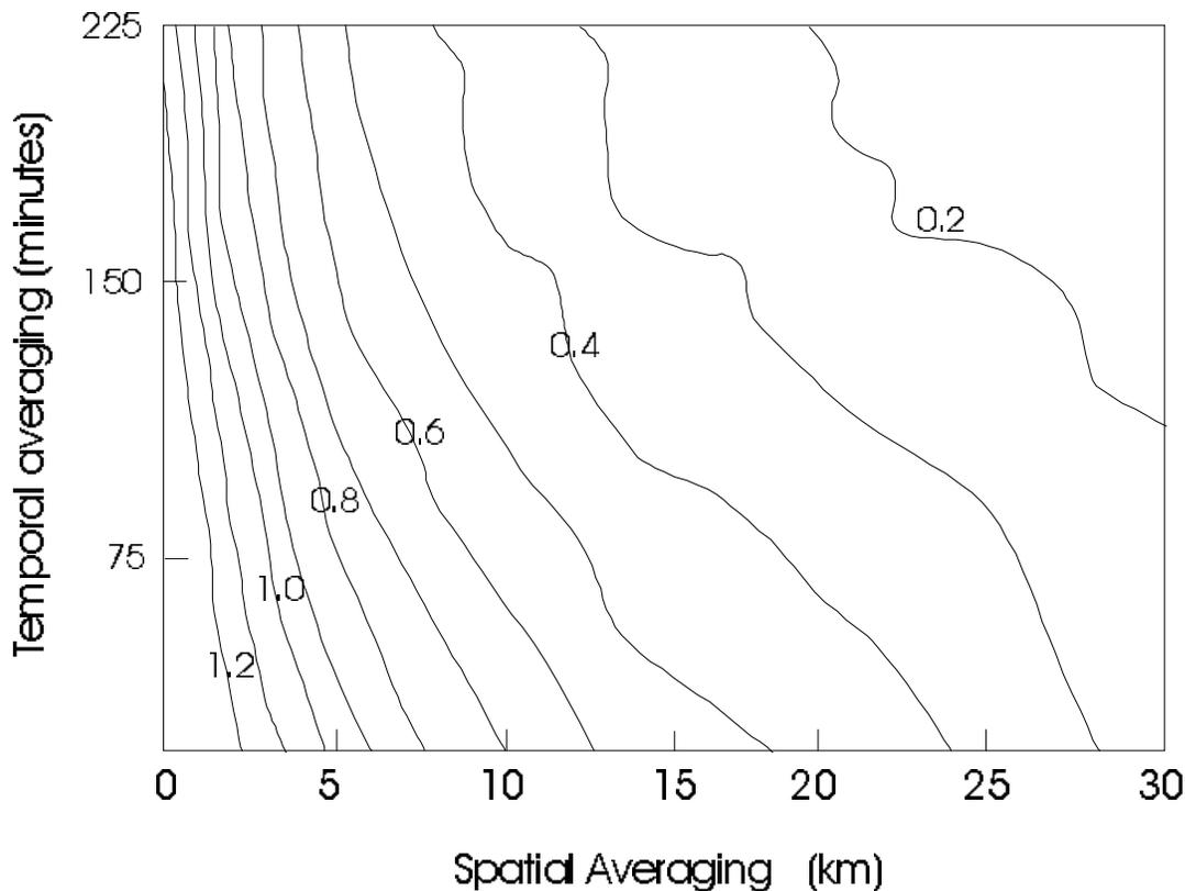
Figure 3: Ratio of the variance to the domain average of the precipitation in a three-dimensional numerical simulation of radiative-convective equilibrium over a water surface, as a function of space-time averaging. The ordinate is the length of time averaging; the abscissa is the length of averaging in space. This ratio asymptotes to  $\sqrt{2}$  for short averaging intervals. (From Islam et al., 1993.)
