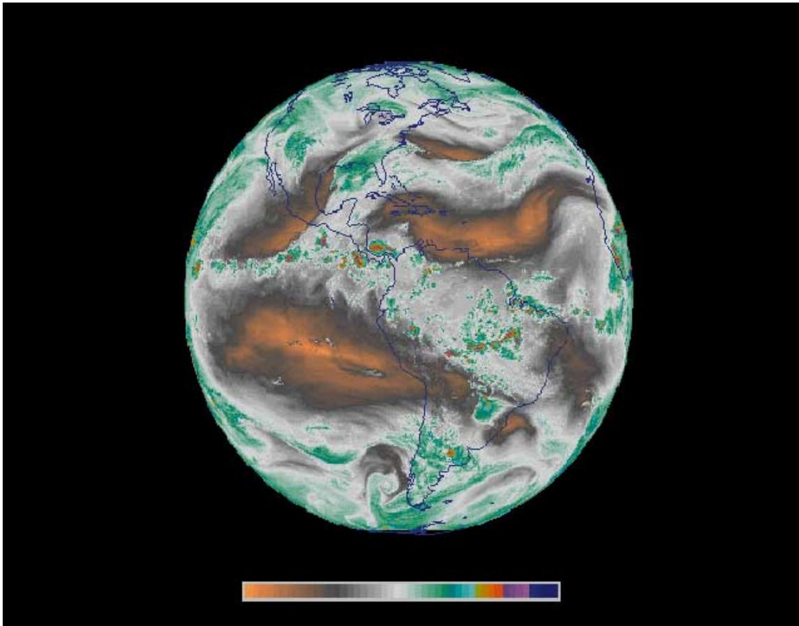
Figure 5: Upper tropospheric humidity patterns on April 27, 1995, at 1745 UTC as measured by the GOES 8 satellite. The 6.7  $\mu\text{m}$  data are related to water vapor, with a peak signal between about 550 and 350 mb. The data are influenced by high clouds. (Image courtesy of A. Gruber and R. Achutuni, NOAA National Environmental Satellite Data and Information Service.)
