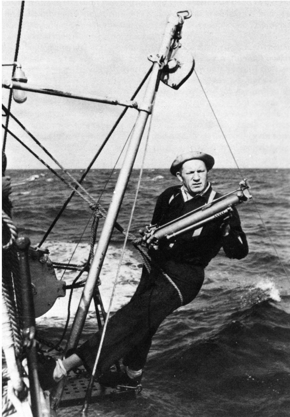
Hanging a Nansen bottle on a wire before lowering it into the sea.
